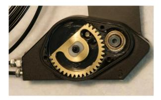
6 Install the small gear on the hexagon of the Rohloffs external gear mech:
