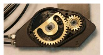
Reinstall the cover on your psh'R-converter and attach it with the attachment-screw to your Rohloff Speedhub.
