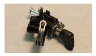
5 Mark the upper Hose on the thumb shifter with scotch-tape and unscrew both hoses from the thumb-shifter.
